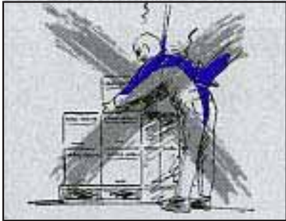
Leaning over the pallet to load and unload boxes on the far side.
