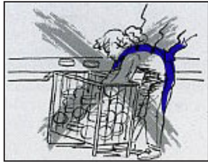
Repetitive bending is required to empty components out of a crate and on to a conveyor belt.
