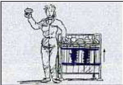
A spring-loaded base keeps the components at a convenient height.
