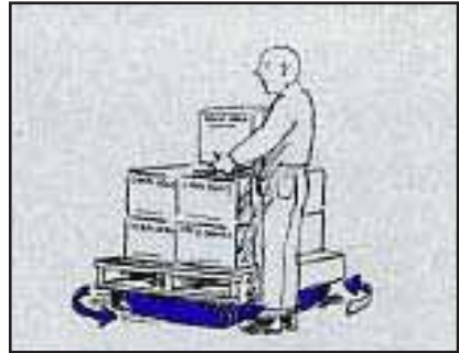
A pallet hoop turntable allows the pallet to be rotated 360° and reducing the carrying or bending required — also providing toe space, to allow the load to be kept closer to the body.
