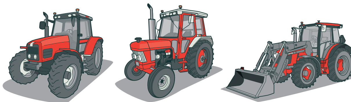
FIGURE 14: Four-wheel drive tractor, two-wheel drive tractor and four-wheel drive tractor with a Front End Loader (FEL)
