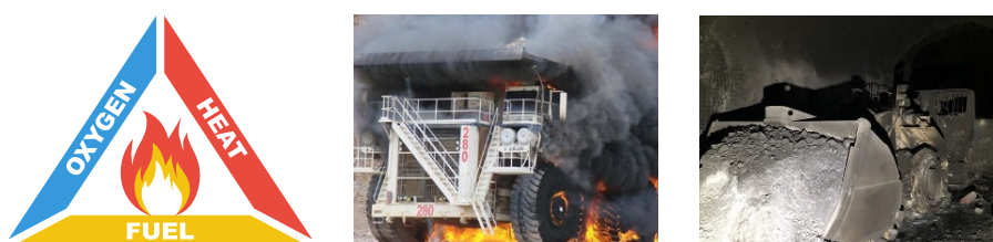
FIGURE 8: The fire triangle and fires at extractive sites
