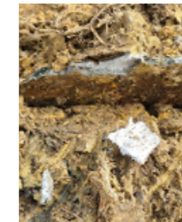
Fragment of asbestos cement pipe and buried cement pipe
