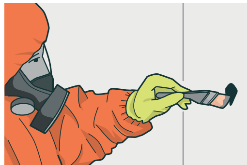
FIGURE 4: Seal drilled edges with sealant
