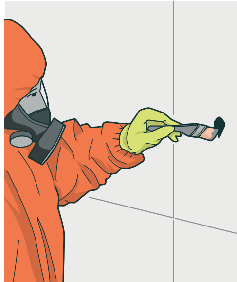
FIGURE 5: Seal drilled edges with sealant
