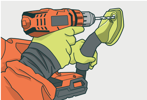
FIGURES 2 AND 3: Drilling hole using chosen method to capture dust
