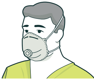
Disposable half facepiece particulate P2 respirator
