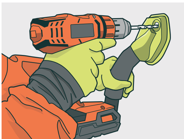
FIGURE 9: Example of using a dust shroud and low speed drill
