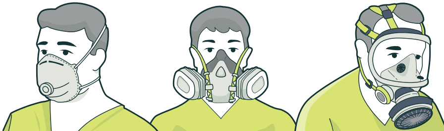
FIGURE 43: Examples of respirators suitable for lower risk asbestos work
