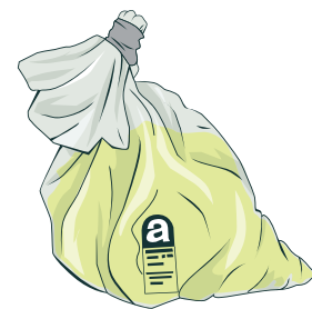
FIGURE 29: Asbestos waste double bagged and sealed with a goose-neck twist
