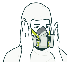
FIGURE 46: Negative-pressure seal check procedure
