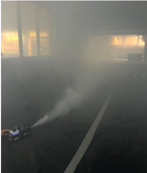
FIGURE 20: An enclosure being smoke tested
