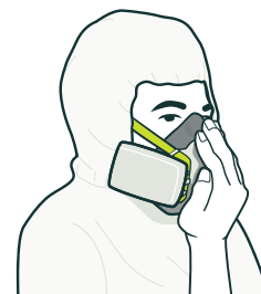
FIGURE 47: Positive-pressure seal check procedure
