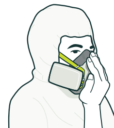
FIGURE 47: Positive-pressure seal check procedure
