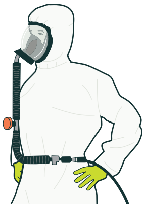
FIGURE 45: Full-face, positive-pressure demand air-line respirator
