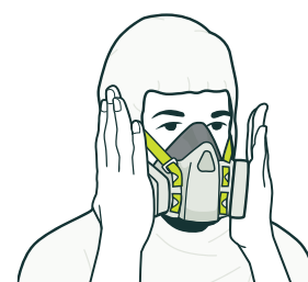
FIGURE 46: Negative-pressure seal check procedure
