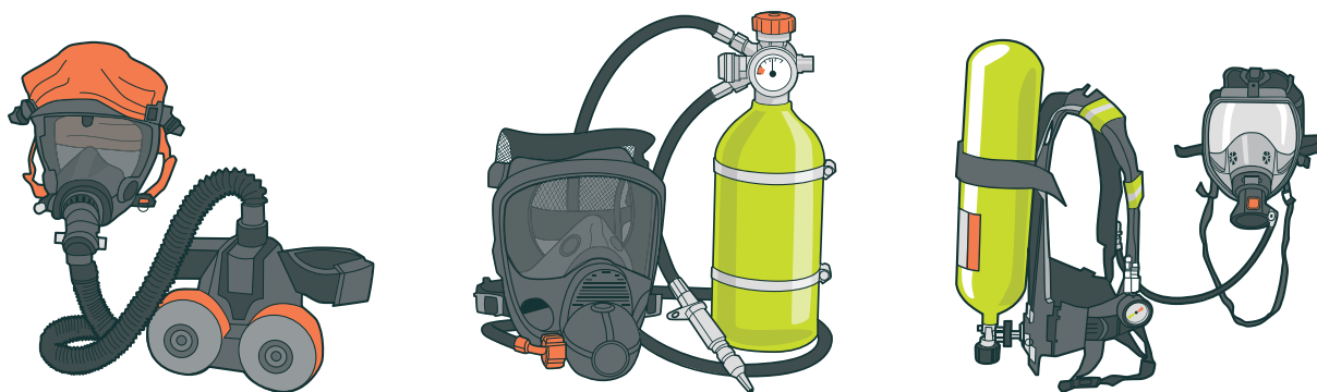
FIGURE 17: Examples of respirators suitable for high-risk assessor work
