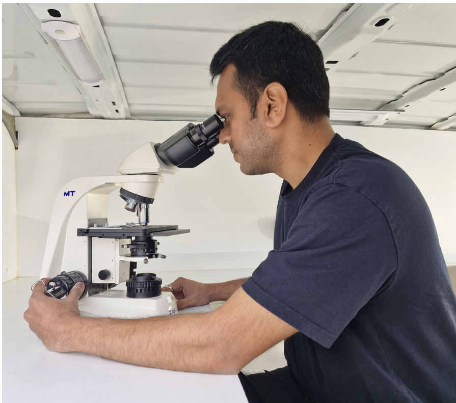
FIGURE 7: Assessor carrying out a PCM count in a mobile laboratory
