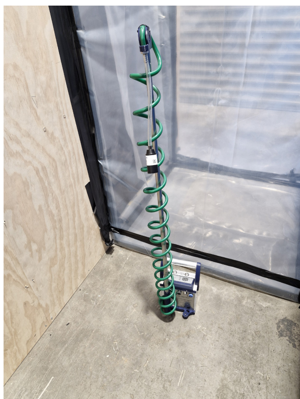
FIGURE 4: Leak test outside an airlock
