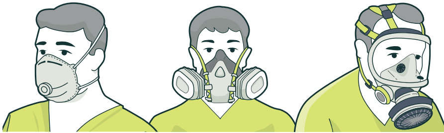
FIGURE 16: Examples of respirators suitable for low-risk assessor work
