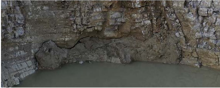
FIGURE 10: Clay pocket within limestone geology
