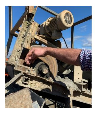
**FIGURE 12:** Photograph of tail drum involved in the incident
