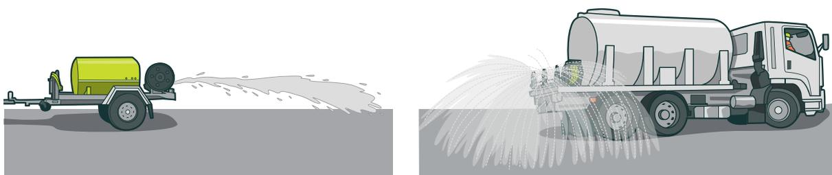
**FIGURE 9:** Examples of using water to dampen dust at unsealed worksites
