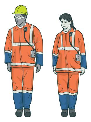
FIGURE 14: Example of workers wearing personal monitoring devices
