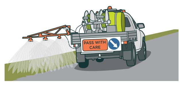
**FIGURE 11:** Example of automated spraying system to limit worker exposure to the chemical being used (also keeps worker in a safer location inside the vehicle)
