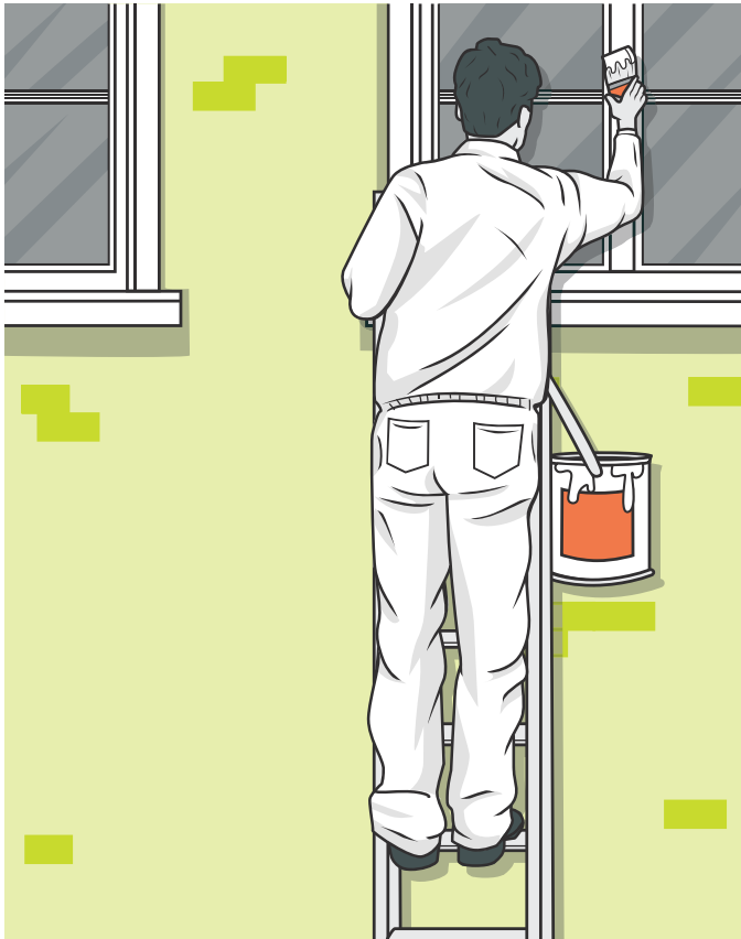
FIGURE 21: Worker maintaining three points of contact with the ladder
