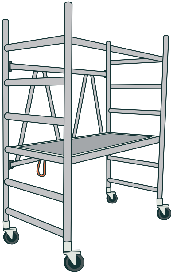
FIGURE 17: A mobile scaffold/ mobile working platform.
