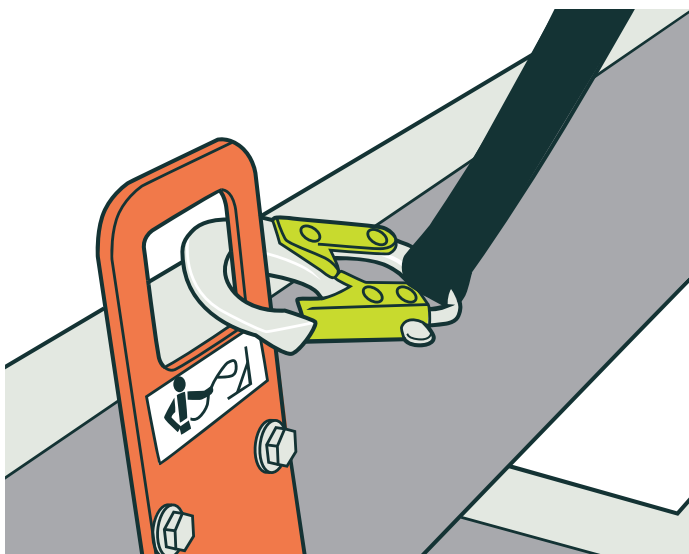
FIGURE 11: Example of correctly placed lanyard connection
