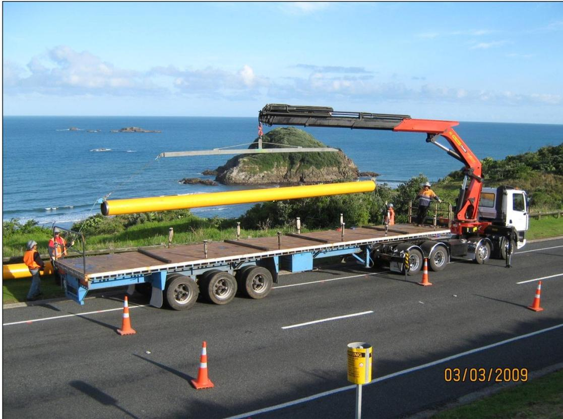
**Picture 6: Truck Loader Crane**
