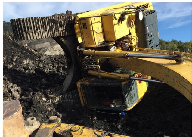
**INCIDENT 3:** An excavator crossed a small culvert onto unlevelled ground with the bucket elevated, causing the excavator to tip over
