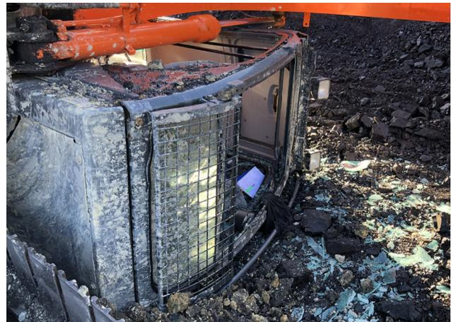
**INCIDENT 2:** The excavator tipped over a one-metre high face/canch. A lone operator had placed his tracks close to the canch edge and was trying to remove a parting. The bucket grabbed and pulled the excavator over the edge
