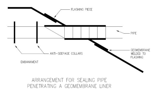
Example of a pipe penetration through earthen compound wall (existing retrofit)
