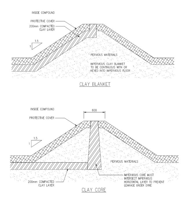
Example of Protecting and Anchoring a Liner
