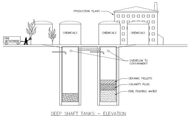
Another option where suitable surface areas are not available. This utilises concrete pipes up to 5 metres diameter and 18 metres deep. The ceramic pellets act like a floating roof, minimising the exposed surface area and thereby reducing vapourisation.
