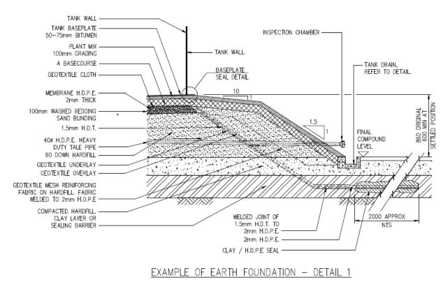
The continuation of the compound floor sealing under the foundation pad is an important detail. Over time, the loads upon the tank foundation tend to cause settlement of the original base resulting in a cone down effect. This may result in tension cracks in a compacted compound floor.
