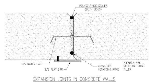
Fire retarding rope is to be placed on both sides of an internal compound wall and may be placed on the internal side only of an external wall.
