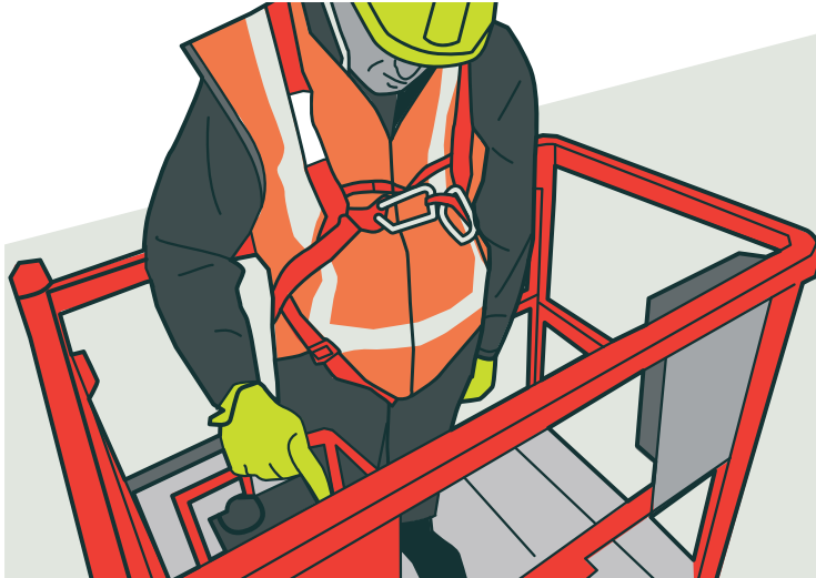
FIGURE 12: A worker restrained in a boom-style elevating work platform
