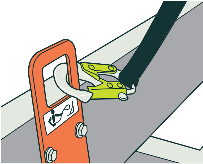
FIGURE 17: Example of correctly placed anchor point
