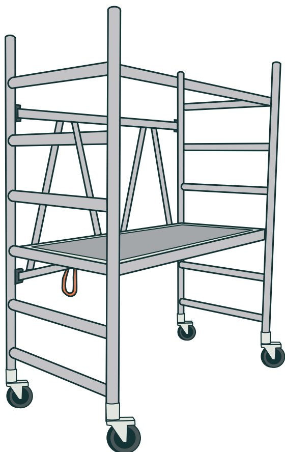
FIGURE 19: A mobile scaffold/ mobile working platform.
