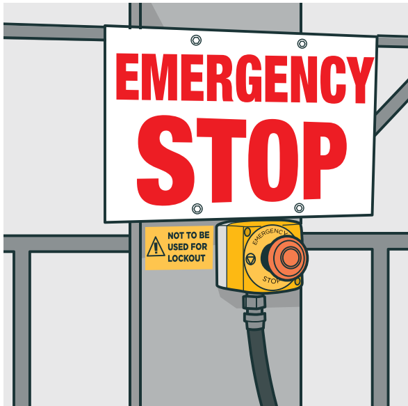
FIGURE 105: Emergency stop with signage
