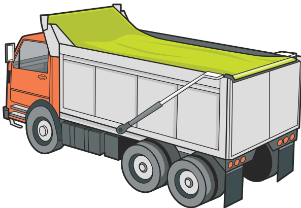
FIGURE 75: Automated covering system
