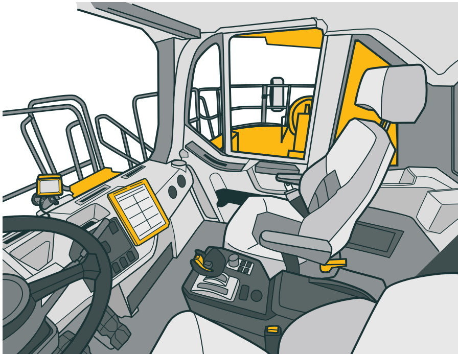
FIGURE 80: CCTV monitor in vehicle cabin
