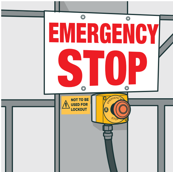
FIGURE 105: Emergency stop with signage
