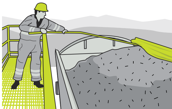
FIGURE 77: Platform covering system
