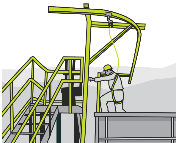
FIGURE 78: Overhead gantry harness system
