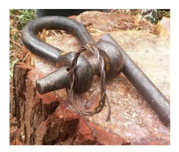
The Knock-Out Pin Shackle used to secure the Madill 171 skyline to the anchor stump
