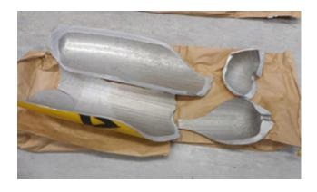
dents or damaged fittings, and if in doubt, do not fill the cylinder.
