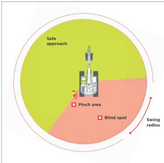
Figure 49: Safe approach zone for an excavator
