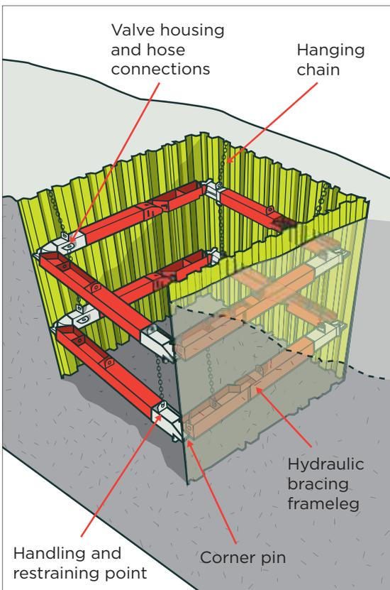
Figure 33: Hydraulic bracing frame with steel trench sheeting
