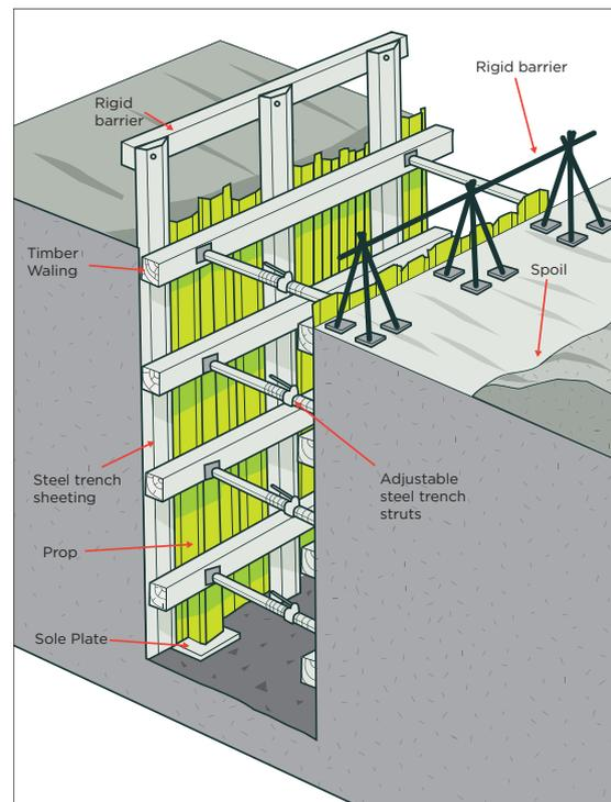
Figure 36: Timber shoring with steel trench sheeting
