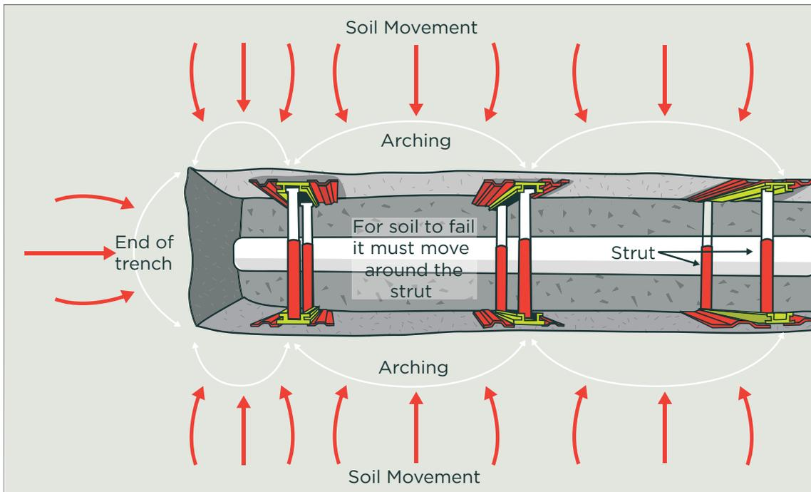
Figure 24: Hydraulic soldier shoring using soil arching
