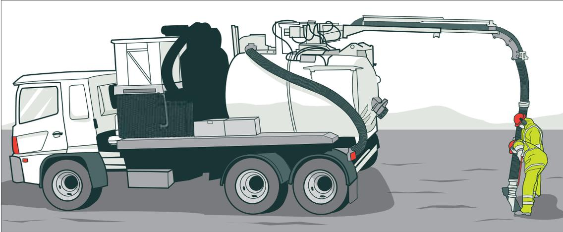
Figure 42: Vacuum truck digging a pilot hole
