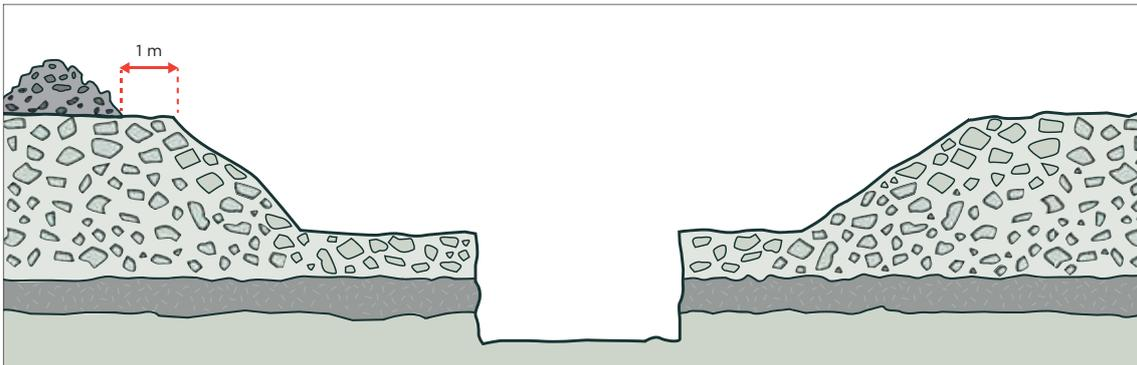
Figure 22: Combination of benching and battering controls
