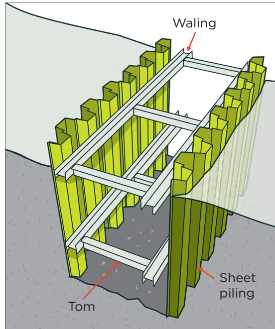
Figure 29: Steel sheet piling with internal waling support
