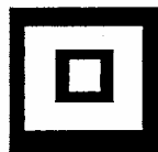
FIGURE 1: DOUBLE INSULATION SYMBOL
