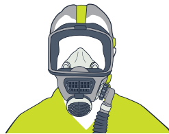
Figure 4: Full-face powered respirator (cartridge)
