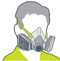
Figure 2: Re-useable half-face respirator (cartridge)
