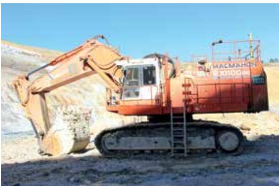
**Figure 93:** This excavator has a good access system, with platforms, guardrails, kick plates and ladder. The ladder is interlocked so the vehicle cannot be started without the ladder being raised (photo courtesy of Newmont Waihi and MacMahon)
