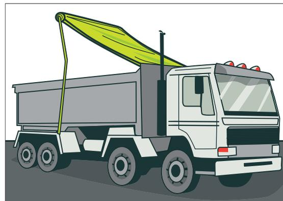
Figure 95: Automated covering system
