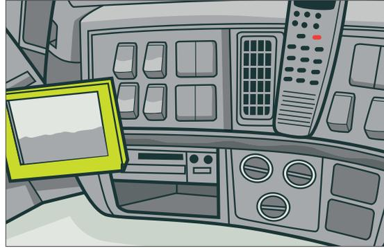
**Figure 63:** CCTV monitor in vehicle cab
