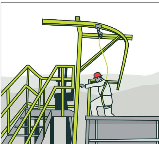
Figure 98: Overhead gantry harness system
