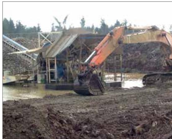
**Figure 52:** Digger and floating screen
