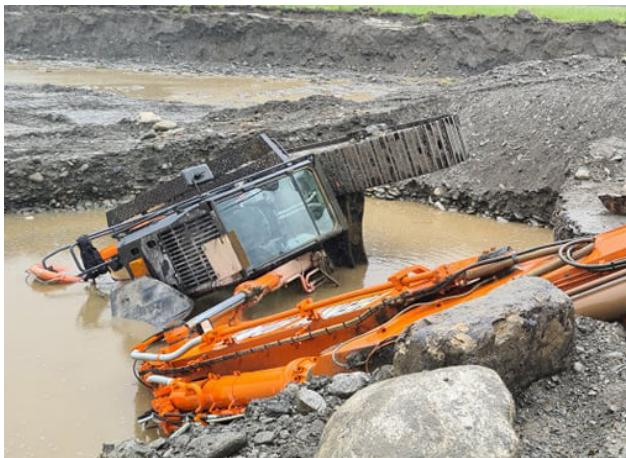
**INCIDENT 4:** The excavator was tramping beside a mine pond when the ground gave way. The excavator track dropped down and the excavator tipped into the pond
