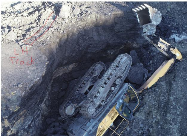
**INCIDENT 5:** The operator positioned an excavator close to the bench edge above an overhang which collapsed due to the machine's weight. The excavator fell approximately four metres
