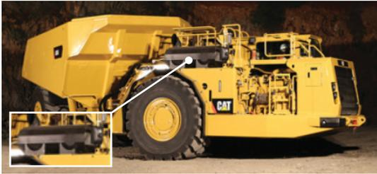
Figure 15: Diesel particulate filter
