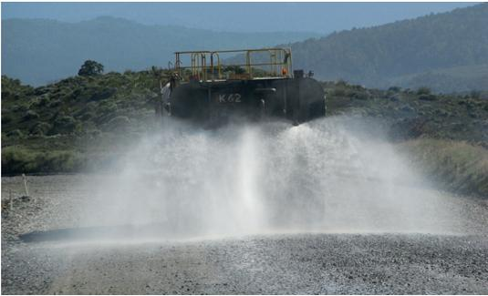
**Figure 4:** Dust suppression using a mobile tanker
